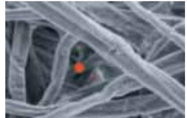
Red circles represent the diameter of a 2-micron and a 5-micron particle.
