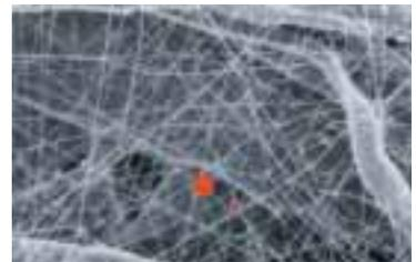
Nanofibers have submicron diameters and small interfiber spaces, which result in more contaminants being captured on the surface of the media and lower restriction.
