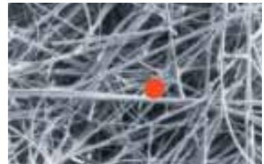
*Red circles represent the diameter of a 20-micron particle.*
